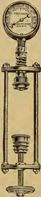
FIG. 111.—Testing Gauge for Syphons.
